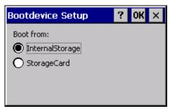
BootDevice Setup is used to specify the medium from which the panel is to start. The relevant selection options are displayed according to the features of the panel.
